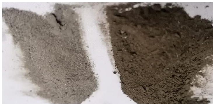
Figure 18. Appearance of the stone dust SD (left) constituent and the synthesized composite BPSD (right) (Ganea & Nan, 2023b)
