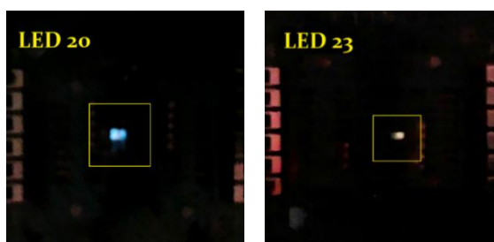
Figure 4.6: left (ITO/PEDOT-PSS/PolyTPD/ CDs-PDA-F3 /Al configuration of LED 20 ) and right (ITO/PEDOT-PSS/PolyTPD/ CDs-PDA-F3 (UV-O 3 )/Al configuration of LED 23 )
