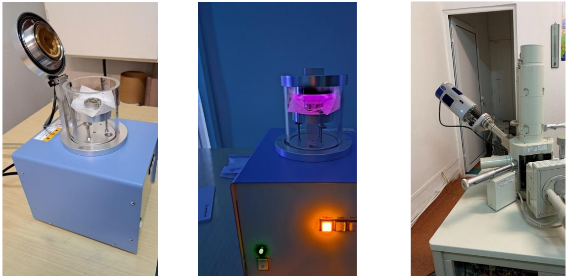
Fig. 2.4. a) Sample preparation for SEM analysis b) SEM JEOL JSM 5600LV microscope with scanning.
