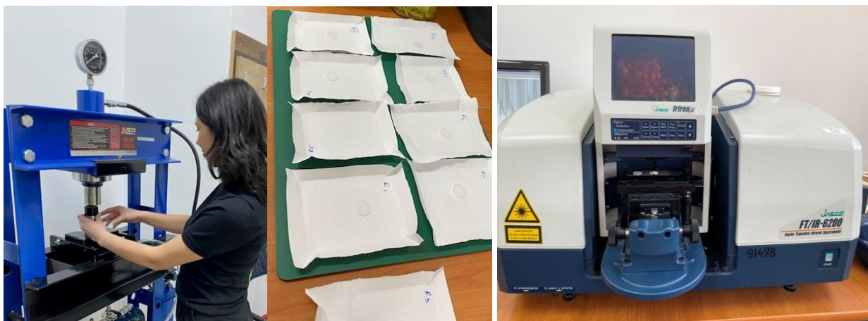
Fig. 2.2. a) Sample preparation for FT-IR spectroscopy measurements and (b) Jasco 6200 FT-IR spectrometer used in experimental studies.
