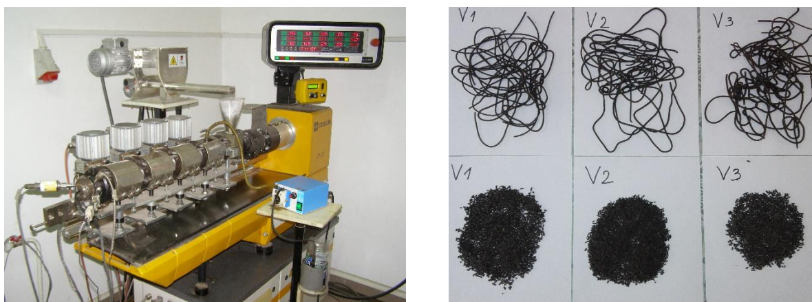
Fig. 1.2. a) Device for the production of organo-mineral fertilizers based on biosolids located at INMA Bucharest Cluj-Napoca Branch and b) organo-mineral fertilizers based on biosolids (V1, V2, V3) produced by INMA Bucharest Cluj-Napoca Branch [13, 14].
