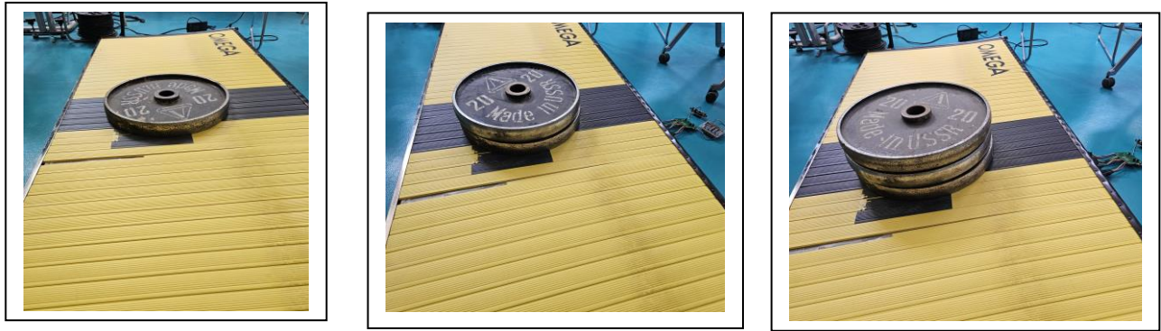
Figure no. 10 - Calibration of the technical solution using disks of 20 kg weight
