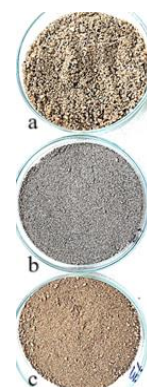
Fig. 5.10 Substrates of sand and tailings: a) Sand; b) St No ; c) St Ox
