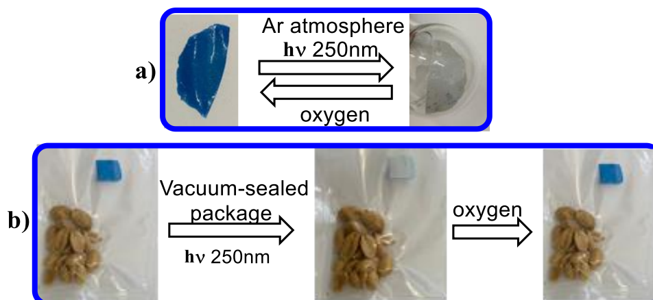
Figure 7. The reversible chromogenic process for photochemical Oxygen-indicators containing titanium dioxide, glycerol, polyvinyl alcohol and phenothiazinium dye: a) MB , b) MBA 2 .
