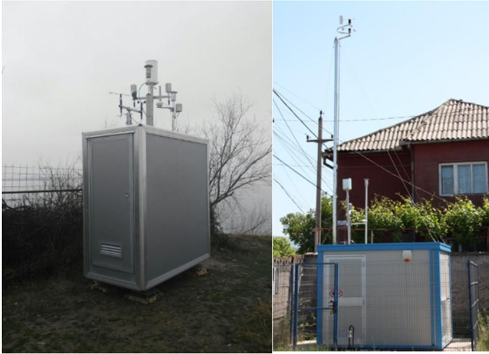
**Figure 2.8:** CS5 air quality station (left) and CS3 air quality station (right) of the Romanian national air quality monitoring network (RNMCA) used during in-situ monitoring around the closed Moldova Nouă tailings ponds, Romania
