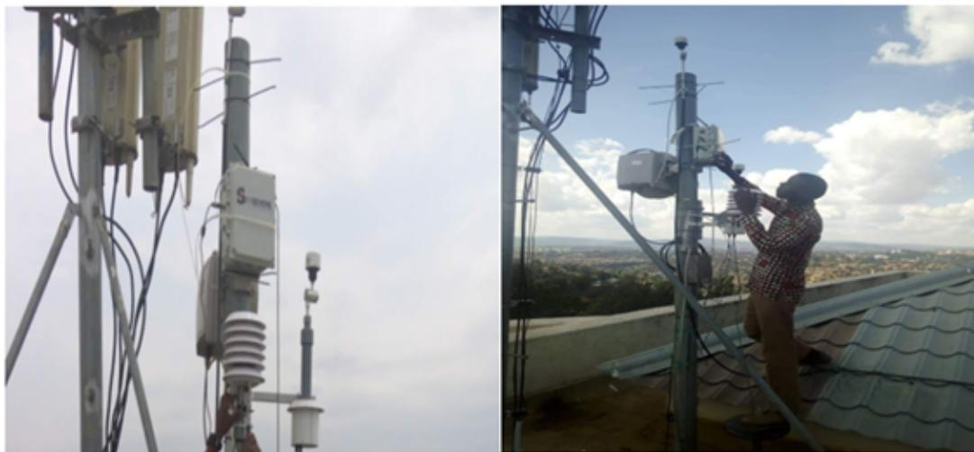
**Figure 2.5:** The thesis author making maintenance of RAMP installed at discrete receptor R3 (left) and at discrete receptor R6 (right). The picture was taken during field monitoring activity
