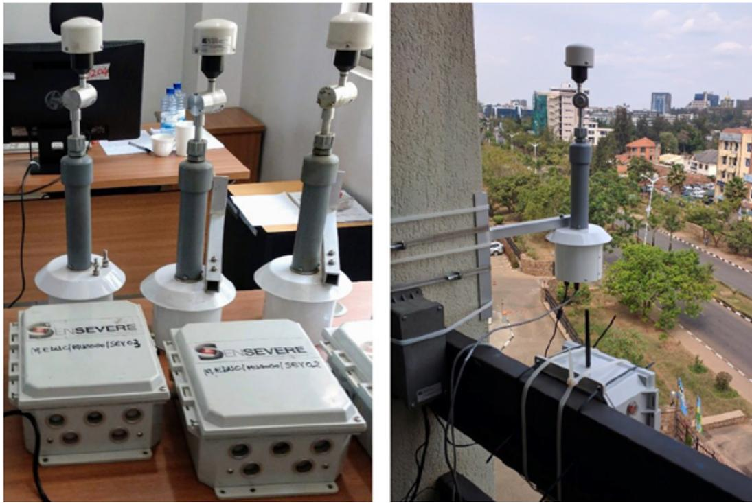
**Figure 2.4:** Real-time affordable multi pollutant (RAMP) air quality monitors in the laboratory for adjustment and maintenance (left) and the installed RAMP for in-situ monitoring road-side target (right). Picture taken by Subramanian et al. (2020)
