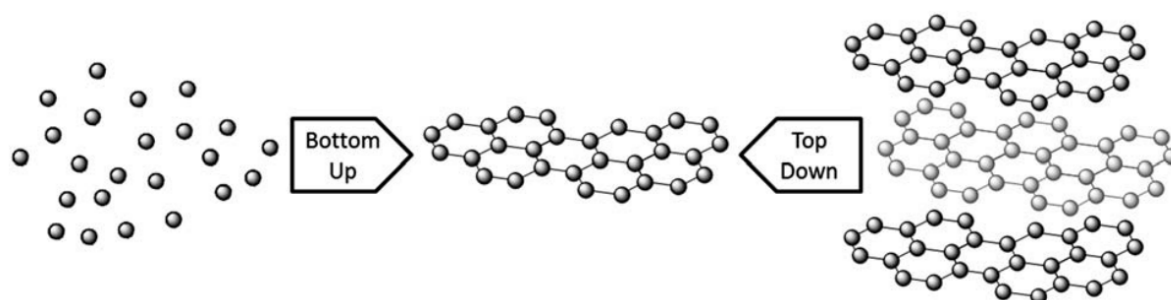
Figure 1.2.1. Simple scheme of bottom-up and top-down approaches in graphene synthesis. Reproduced with permission from [3].
