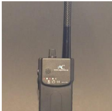
Figure 3 AC system transmitter
