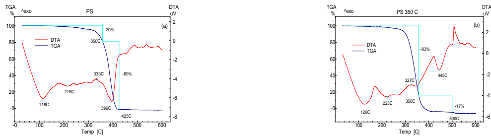
Figure 4.2. DTA / TGA curves for: (a) unheated polystyrene ( PS) and (b) polystyrene heated to 350 °C ( PS 350 °C).
