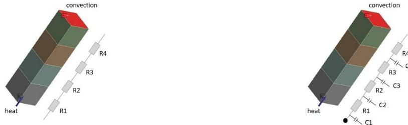
**Figure 3.** Representative view of a one-dimensional heat path
