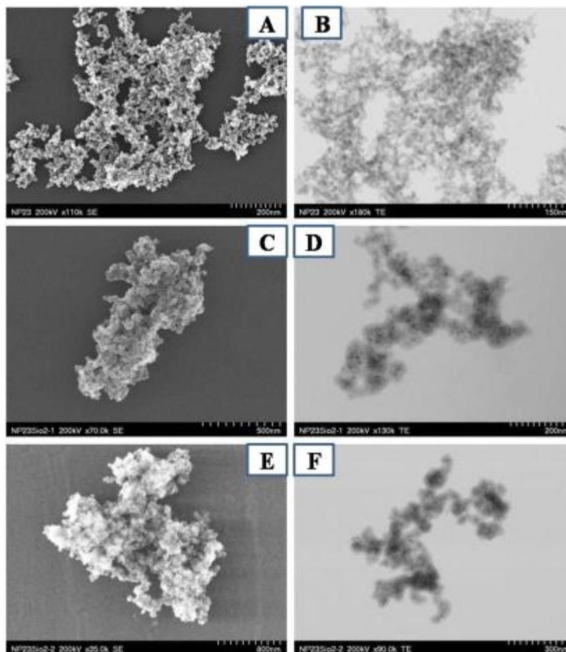
**Figure 1.** SEM and TEM images of magnetic nanoparticles (MNPs) and SiO<sub>2</sub>-coated magnetic nanocomposites (MNPs): **A** (SEM), **B** (TEM) uncovered magnetic nanoparticles; **C** (SEM), **D** (TEM) for magnetic nanocomposites MNPS- SiO<sub>2</sub>-1; **E** (SEM), **F** (TEM) for the magnetic nanocomposite MNPS- SiO<sub>2</sub>-2.
