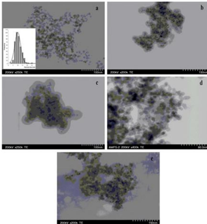
**Figure 4.** The morphology of the MNPs (a) and MNPs coated with SiO<sub>2</sub> shell, MNPs-SiO<sub>2</sub> (b) and polymer-coated MNPs MNPs-SiO<sub>2</sub>-pAAc (c), MNPs-SiO<sub>2</sub>-pAMPS (d) and MNPs-SiO<sub>2</sub>-CHIT (e).
