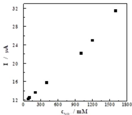
**Figure 6.** Calibration curves for nitrite, as measured using MNPs-SiO<sub>2</sub>-pAAc electrode.
