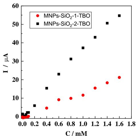
**Figure 3.** Calibration curves for nitrite, as measured using NP-SiO<sub>2</sub>-1-TBO and NP-SiO<sub>2</sub>-2-TBO electrodes
