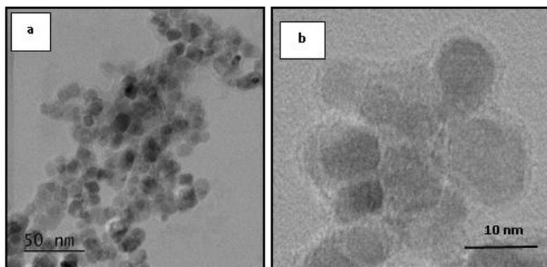
**Figure 7.** TEM microscopy images for magnetic hydrogel nanocomposites (MNP-pAAc) based on cross-linked polyacrylic acid (various magnifications)
