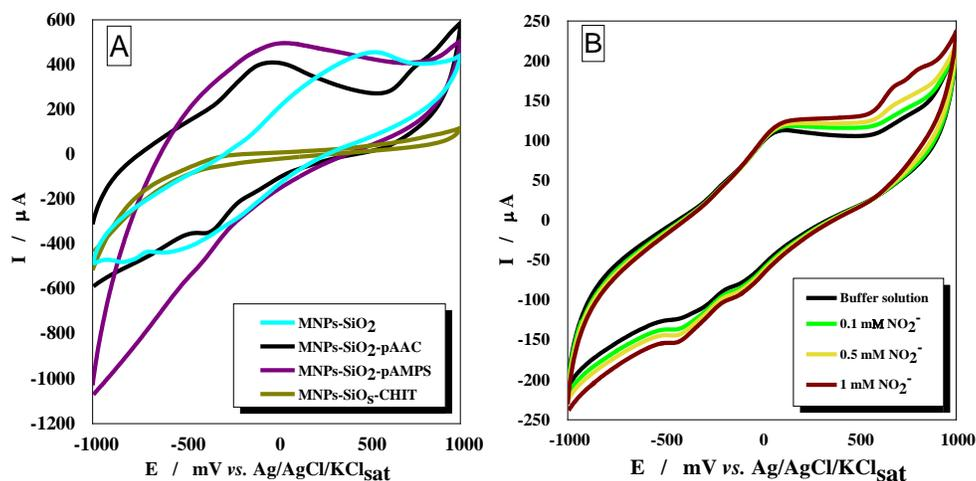
**Figure 5.** (a) Electrochemical response of carbon paste electrodes modified with MNPs-SiO<sub>2</sub>, MNPs-SiO<sub>2</sub>-pAAc, MNPs-SiO<sub>2</sub>-pAMPS, MNPs-SiO<sub>2</sub>-CHIT;
