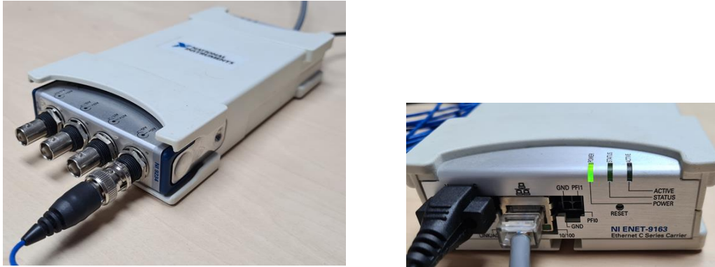
Figure 5.17 Data acquisition and processing system
