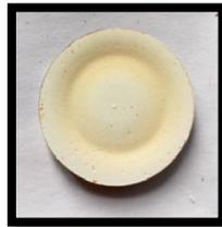
*Fig.3.1.1 Ring-shaped erosion on the surface of the target*
