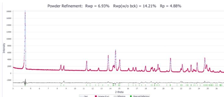
Figure 3.7: Comparison of the experimental pattern with the calculated one
