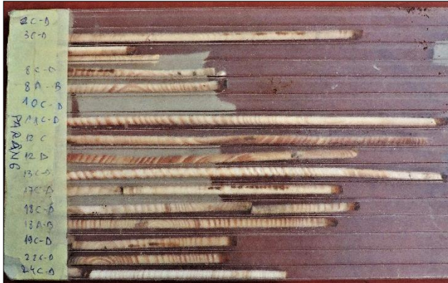
Fig. 10 Increment cores in a polycarbonate sheet
