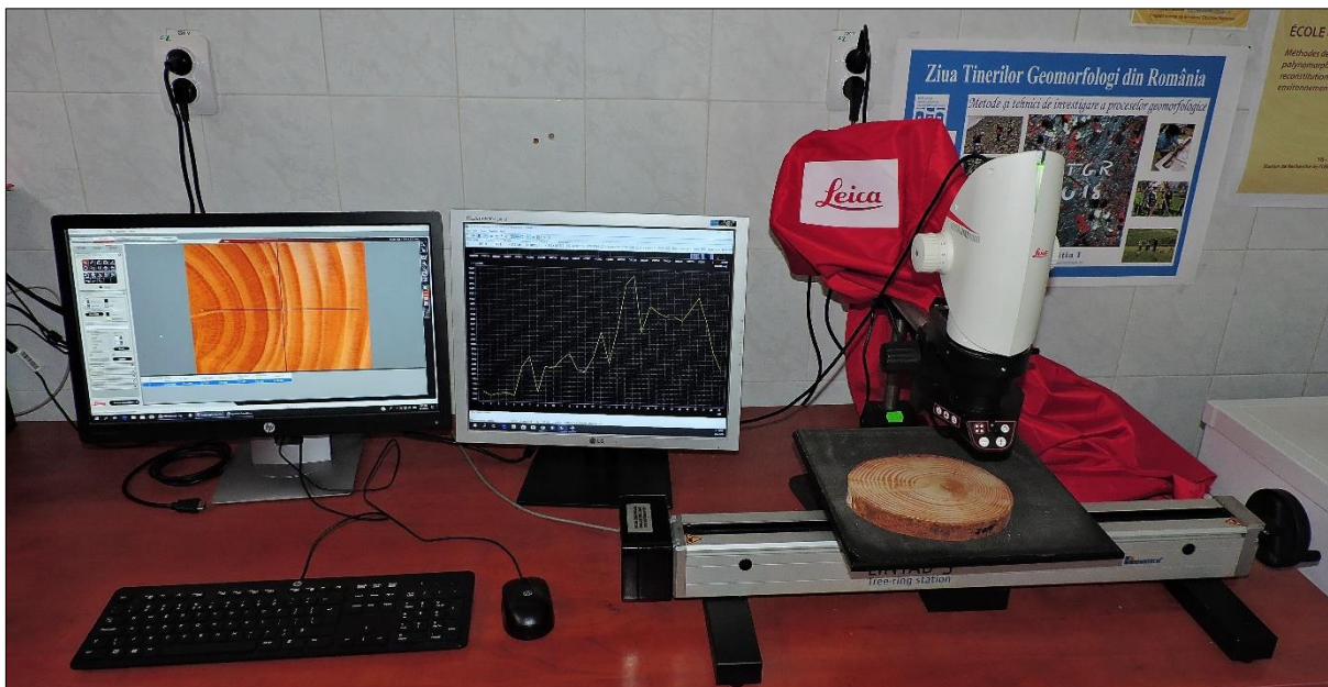
Fig. 11 LINTAB 5 station and the microscope Leica DMS 1000 connected to a computer
