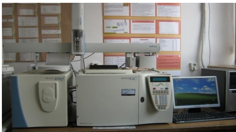
Fig. 4. 4. GC-MS with autosampler.
