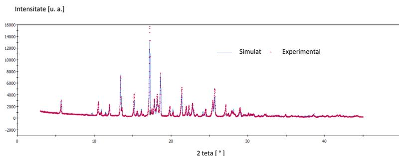
**Figure 4.5** Experimental and calculated diffraction pattern of pitofenone hydrochloride using the Pawley method with SuperNova X – ray diffractometer on monocrystals
