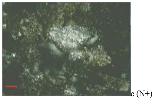
Fig.5.1. Assay I, (52.88% limestone; 7.09% clay; 40.03% gypsum, 1220 °C) , 50 μm
