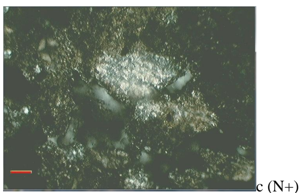
Figura.5.1. Proba1, (52, 88% calcar;7,09% argilă; 40,03% ghips, 1220 0 C) , 50 μm
