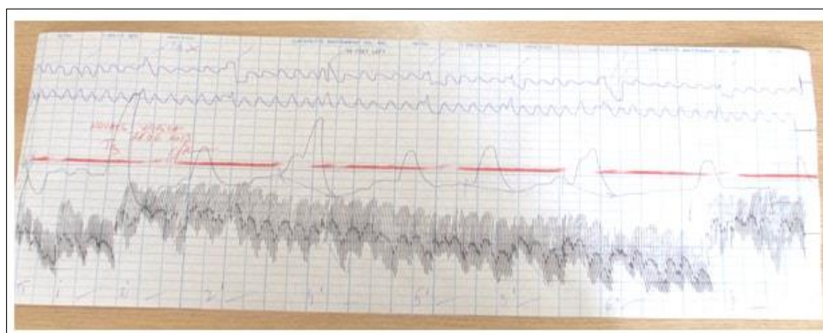
Figure 44. Highlighting the reaction to the verbal stimulus in the physiological plane: Respiratory (thoracic and abdominal - the first two diagrams in blue); Electrodermal (galvanic skin reaction - third black color chart); Cardiovascular (brachial and distal pulse - the last two charts in black).
