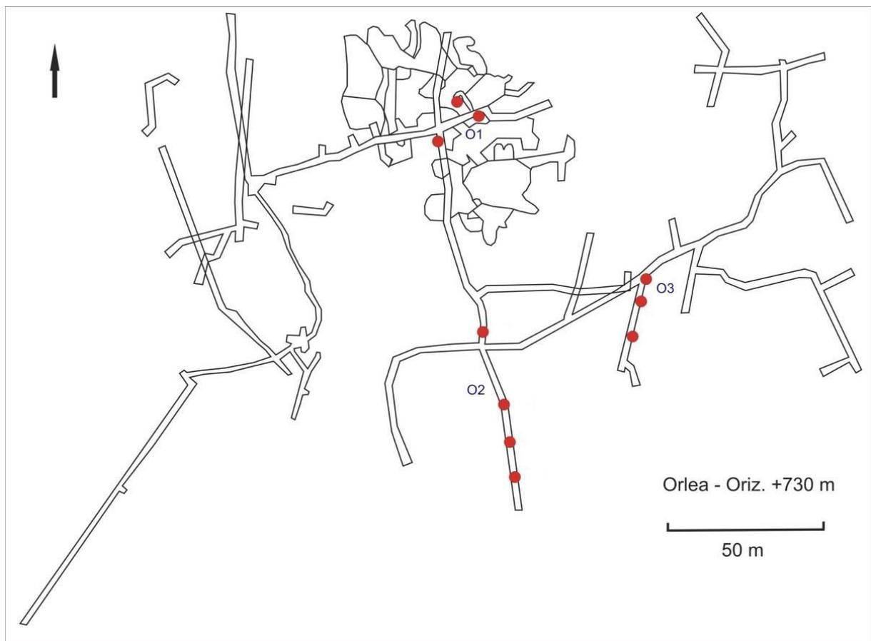
*Fig. 18. Topographic map of the underground mining works from Orlea, +730 level, with the location of sampling areas (RMGC courtesy).*
