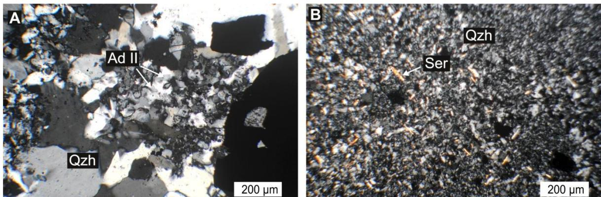
*Fig. 14. Microphotographs in polarized light (two polarizers). A - microscopic view of euhedral adularia II rhombus crystals (Ad II) accompanied by hydrothermal quartz veins (Qzh); B - microscopic view of an intense silicification (Qzh) of the vent breccia matrix associated with a minor phyllic alteration (Ser)(sericite flakes) (Drăguşanu and Tămaş, in print).*
