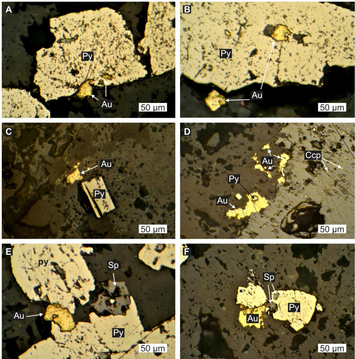
*Fig. 20. Reflected light microphotographs (one polarizer) presenting electrum mineral assemblage from the rhodochrosite vein from +730 level, Orlea mining field. Abbreviations: Au – electrum (gold), ccp – chalcopyrite, py – pyrite, sp – sphalerite.*
