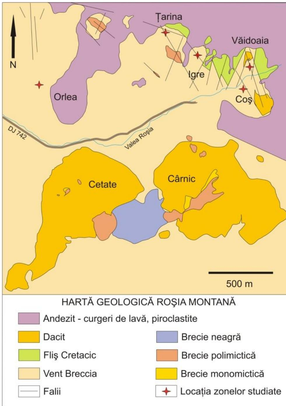
Fig. 1. Geological map of Roșia Montană ore deposit with the main mining fields (RMGC courtesy); the position of the faults is given after Hewson et al., (2005).
