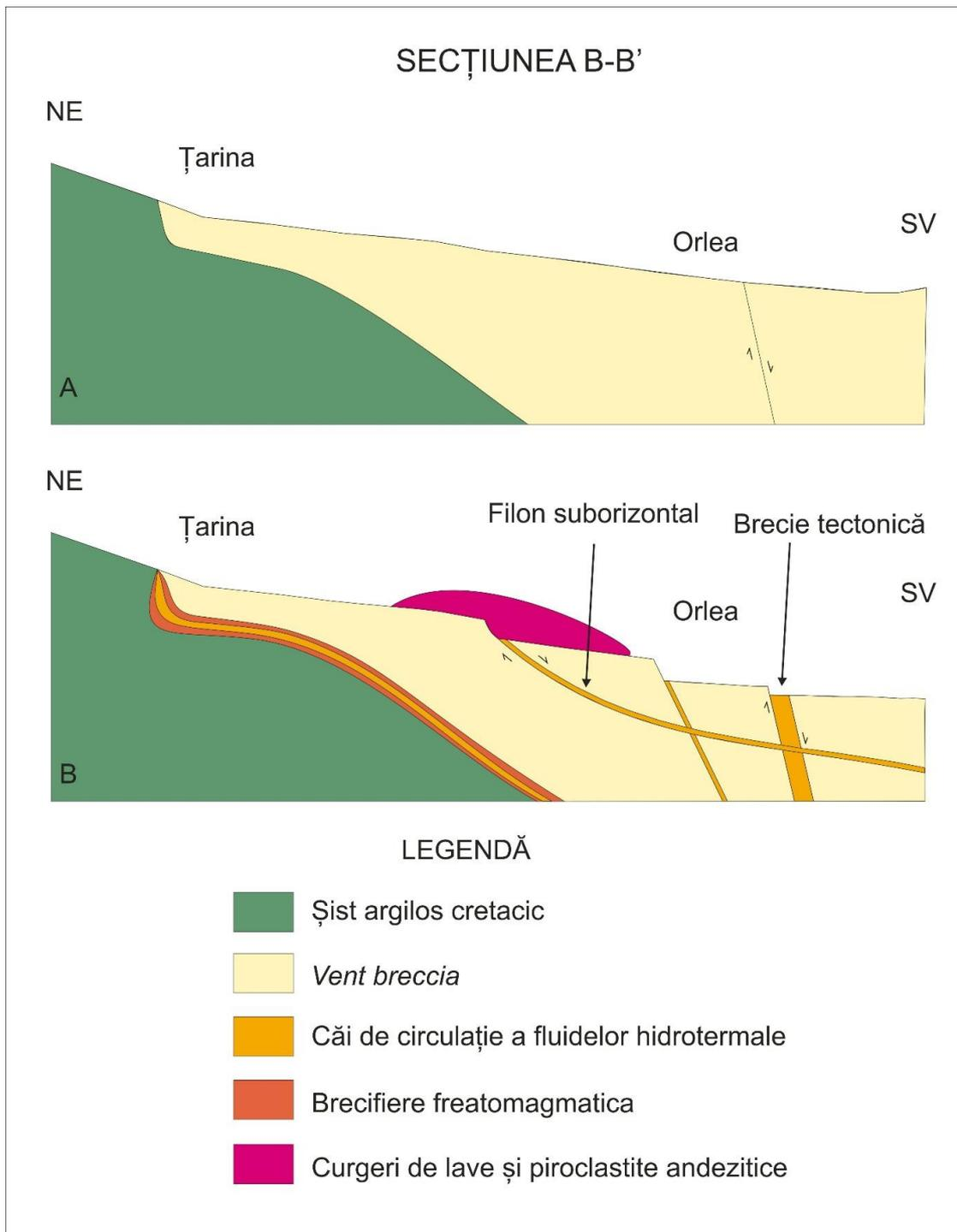
*Fig. 26. Simplified ore deposit model for Țarina and Orlea mining fields. A - The phreatomagmatic breccias were emplaced along the contact vent breccia - Cretaceous basement; B - Hydrothermal fluid flow and ore deposition took place along the above mentioned contact and through regionally and locally controlled faults.*
