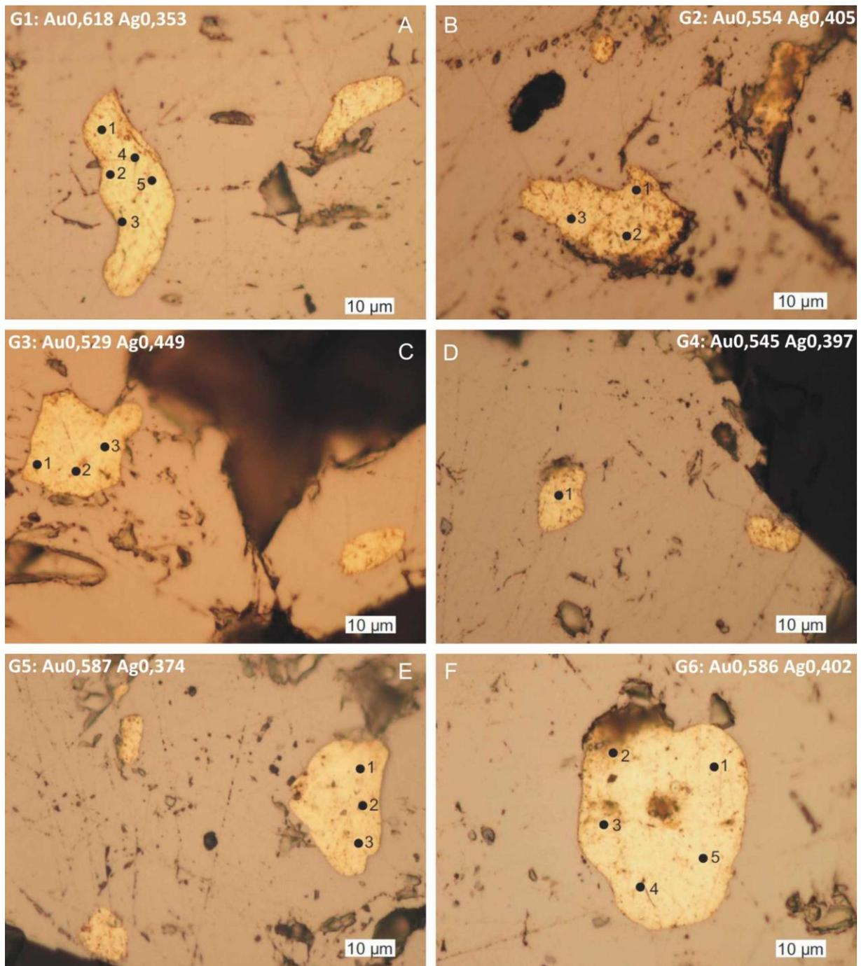
*Fig. 9. Microphotographs in reflected light (one polarizer) showing the electrum grains from Coş mining field analyzed by the means of EPMA; the points and their corresponding number shown in the microphotographs indicate the analyzed points; the mean calculated chemical formula corresponding to the analyzed grain is typed on the upper right corner of each image. All the electrum grains are hosted in pyrite.*
