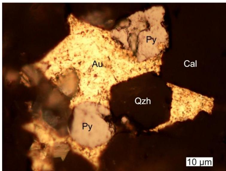
Fig. 16. Microphotograph in reflected light (one polarizer) of electrum (Au) in association with pyrite (Py), calcite (Cal) and hydrothermal quartz (Qzh) (Drăgușanu și Tămaș, in print).
