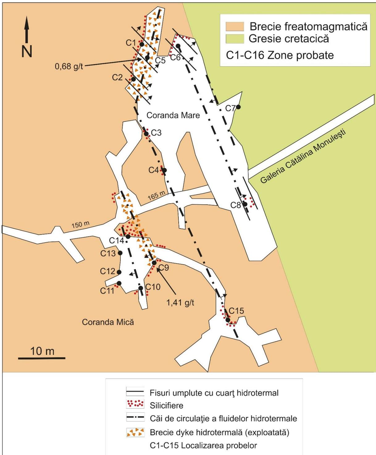
Fig. 4. Underground mining works from Coș mining field (RMGC courtesy) with the location of the sampling zones. The geologic data comprise the lithologies, the hydrothermal fluids flow lineaments, the hydrothermal breccia dyke structures and the silicification accompanying the mineralized zones.
