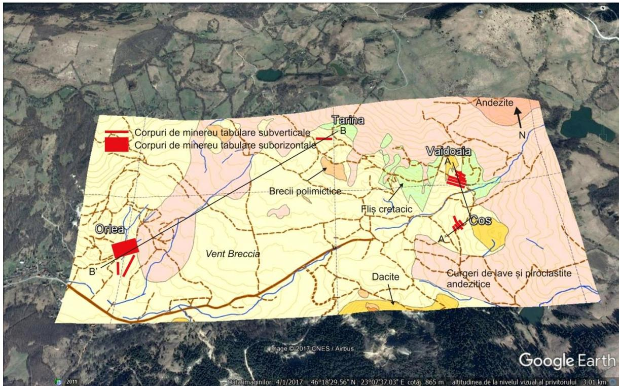
Fig. 24. Georeferencing geological map (RMGC courtesy) in Google Earth of the northern part of Roşia Montană ore deposit with representation of the studied tabular ore bodies.
