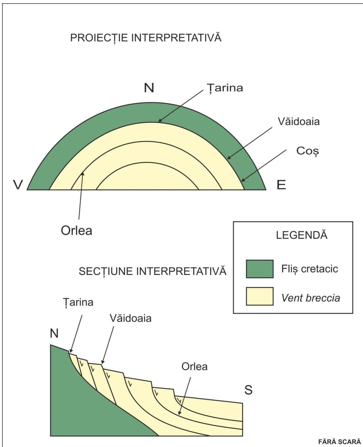
Fig. 23. Interpretative horizontal projection (upper image) and cross section (lower image) of the northern part of Roşia Montană ore deposit, showing the contact between diatreme breccia (vent breccia) and Cretaceous flysch (basement), with the set up of subsidence towards the inner part of the diatreme partly controlled by ring shaped take-off planes similar to listric faults.
