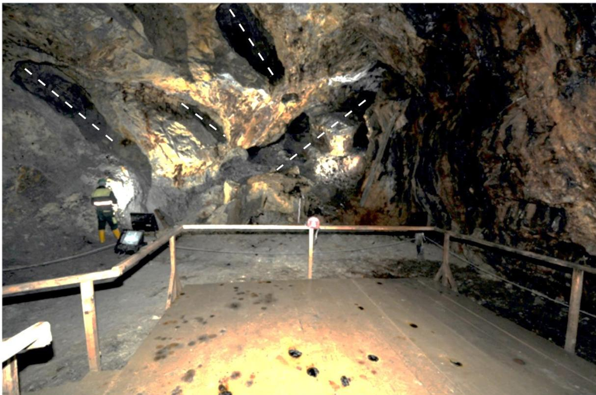
*Fig. 6. Northern face of Coranda Mare stope and the position of hydrothermal breccia dyke structures (dot lines).*
