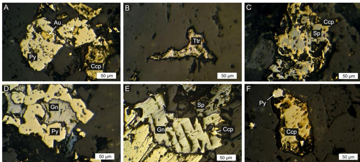
*Fig. 8. Microscopic views of ore minerals identified in Coş mining field. A - electrum in association with pyrite and chalcopyrite; B - tetrahedrite deposited in an open space; C - sphalerite in association with chalcopyrite; D - galena in association with pyrite; E - galena in association with pyrite, sphalerite and chalcopyrite; F - chalcopyrite in association with pyrite; Abbreviations: Au – electrum; ccp – chalcopyrite; gn – galena; py – pyrite; sp – sphalerite; ttr – tetrahedrite.*
