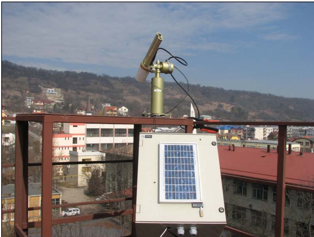
Figure 3.11 - NASA-AERONET #643 Cimel CE 318A sun-photometer Faculty of Environmental Science and Engineering, Babeş-Bolyai University Cluj-Napoca (Ajtai et al., 2012b)
