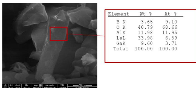
Fig. 5 SEM and EDX results for the sample heat treated for 30 minutes at 900^\circ\text{C}
