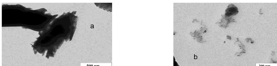
Figure 3.12. TEM images Ni-Cu(1)/Al catalyst: a -150°C; b -350°C
