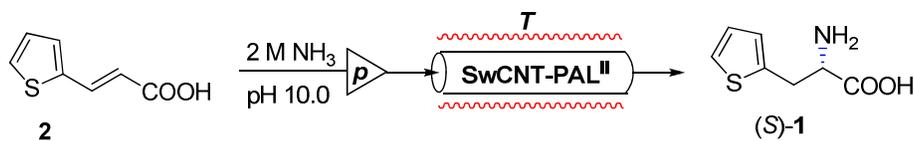
Figure 5 Ammonia addition to 3-(thiophen-2-yl)acrylic acid **2** catalyzed by SwCNT<sub>COOH</sub>-PAL<sup>II</sup> in a continuous-flow packed-bed microreactor (flow 0.1 mL/min)
