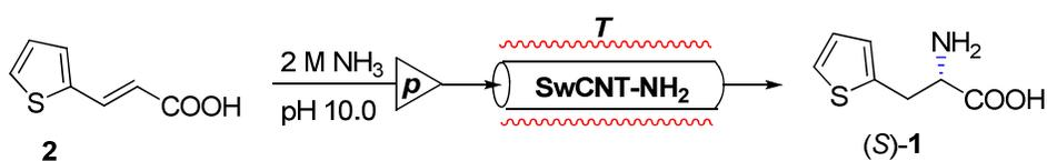
**Figure 7** Ammonia addition to 3-(thiophen-2-yl)acrylic acid **2** (4.5 mM) catalyzed by SwCNT<sub>NH<sub>2</sub></sub>-PAL in a continuous-flow packed-bed microreactor (flow rate: 0.1 mL min<sup>-1</sup>, column: 30 mm × 3 mm ID;).
