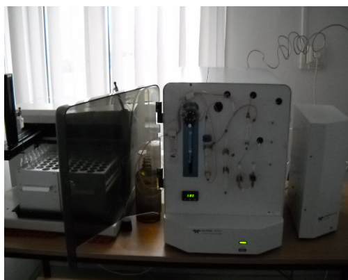
Fig.5.2.1 – Total Organic Carbon Analyzer TOC – Apollo 9000 - Teledyne Instruments
