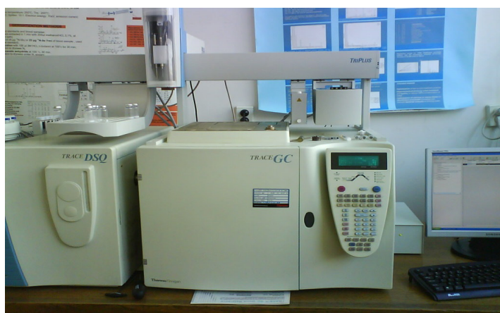
Fig. 2.7. Trace DSQ ThermoFinnigan MS coupled with Trace GC-system equipped with autosampler
