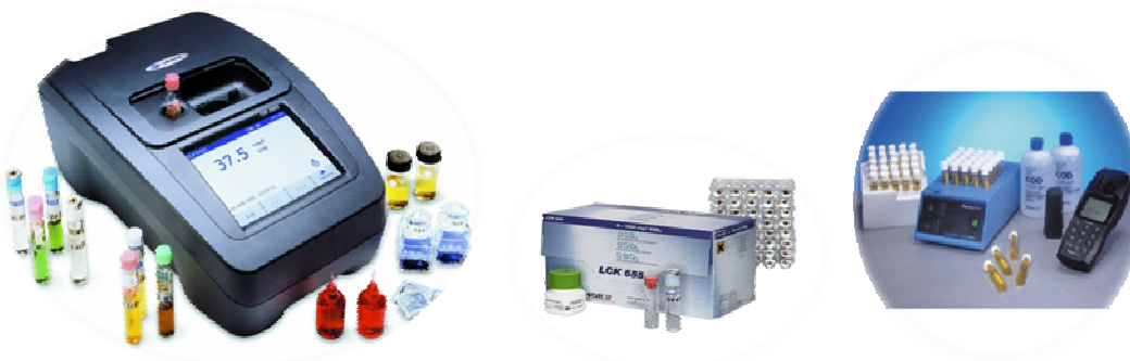
Figure.6.2.1. Spectrophotometer DR HACH 2800, LTV073 thermostat, set for water dilution and cuvette test for determination of BOD 5
