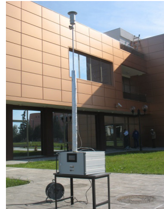
Fig. 5.5.2. A complex system of ICIT Rm. Valcea mobile laboratory, used for in situ monitoring
