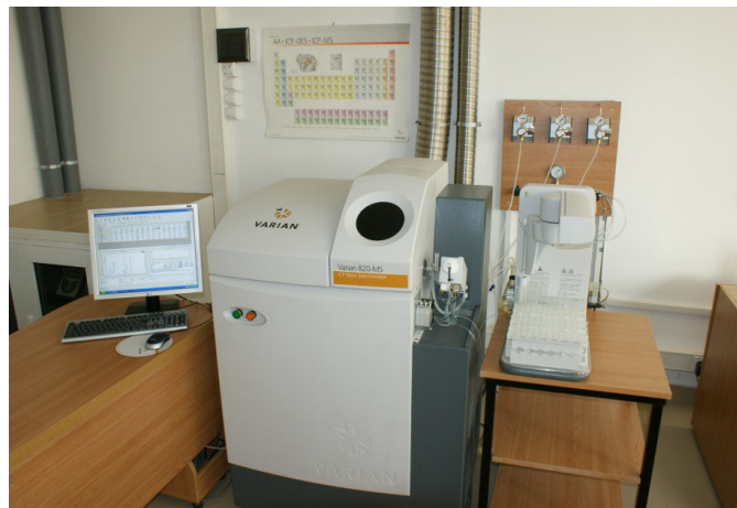
Fig 5.1.7. Inductively coupled plasma mass spectrometer ICP-MS, Varian 820
