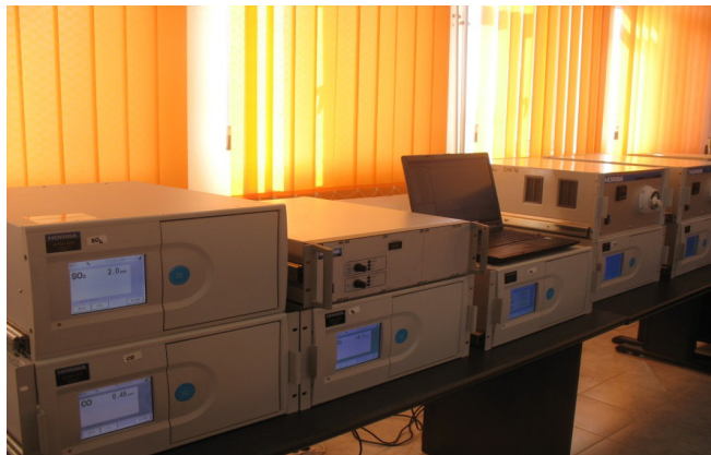
Fig. 5.5.2. A complex system of ICIT Rm. Valcea mobile laboratory, used for in situ monitoring
