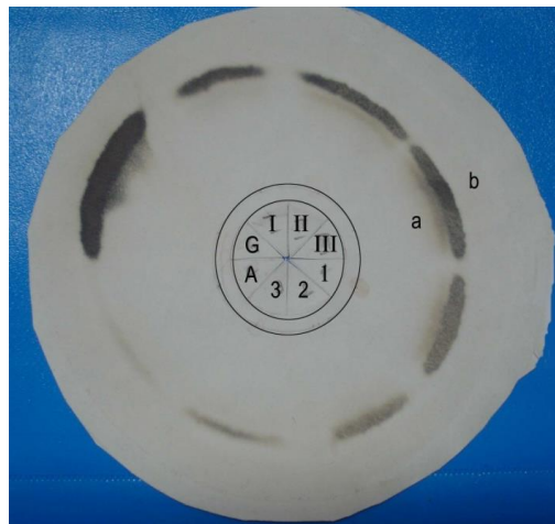
Fig. 29. Amylase activity (AA). 1-3 sediment samples Văliug; I-III sediment samples Secu + enzyme substrate (starch 2%), A=control – starch solution 2%. G=glucose a=amylase spot. b=glucose spot.
