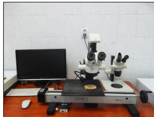
**Fig. 2.** The LINTAB measuring station and Leica stereo microscope
