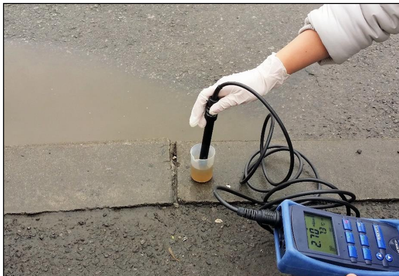
Fig. 8. 1 Onsite measurements with a WTW handheld pH/Cond 340i multi-parameter instrument (Ivan et al., 2016).
