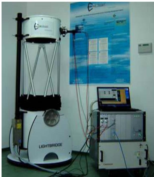
Fig. 3.9. The lidar system at the Faculty of Environmental Science and Engineering, UBB Cluj Napoca
