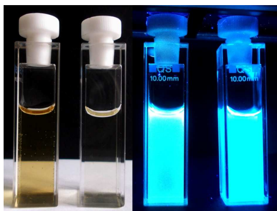
Figure 1. Aqueous solution of CDs-PEG 1500N and CDs-PD under normal light conditions (left) and under irradiation at 365 nm (right)
