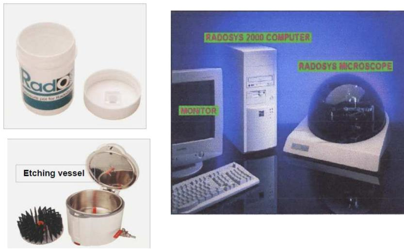
**Figure 4.:** Device RadoSys 2000 (right), the box Radaplot for detector CR-39 (top left corner) device for detectors development (bottom left corner)
