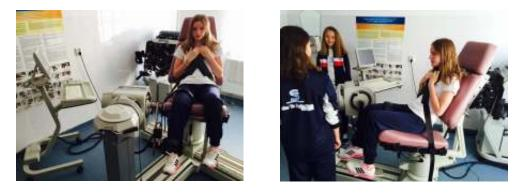
We ran two tests, the first test (T1) was done before the start of the training period and it consisted of 2 maximum isometric contractions for 5 seconds at different angles for each leg separately. We recorded 4 values for each swimmer separately, at 1000 and 1200 angles. The second test (T2) was done after 6 weeks of training.
