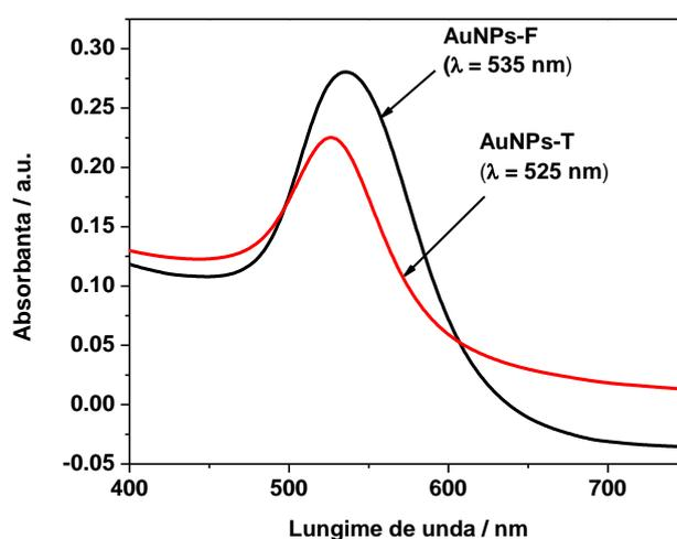
**Figure 2.3** UV-Vis spectra of AuNPs-T and AuNPs-F (1:4 volume ratio AuNPs:H<sub>2</sub>O)
