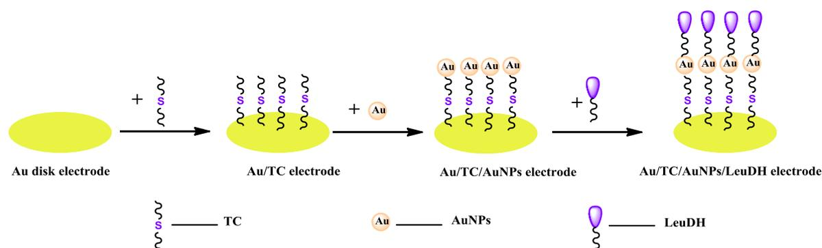
**Figure 4.1** Illustrative representation of leucine dehydrogenase biosensor
