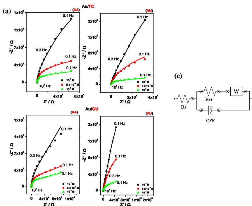
**Figure 3.14** Nyquist plots for: **a** – Au/TC electrode and **b** – Au/GU electrode in PBS solution containing various ascorbic acid/ uric acid concentrations; the continuous lines represent the fit based on the equivalent circuit (b)
