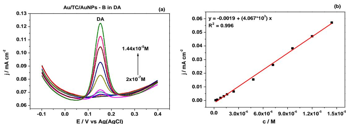
**Figure 3.18 (a)** DPVs recorded for Au/TC/AuNPs-B electrode in pH 7.2 PBS containing DA:  $2 \times 10^{-7}$  –  $1.44 \times 10^{-5}$  M; **(b)** linear response of the modified electrode in the concentration range:  $2 \times 10^{-7}$  –  $1.44 \times 10^{-5}$  M
