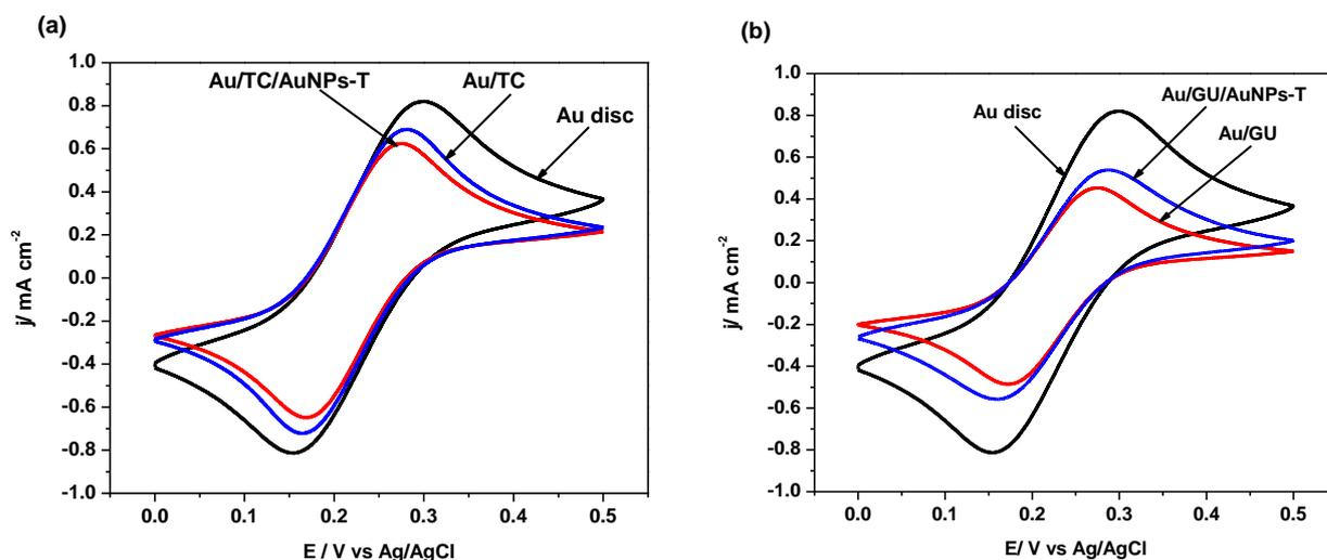
**Figure 2.10** Cyclic voltammograms for (a) Au disk, Au/TC, Au/TC/AuNPs-T electrodes and (b) Au disk, Au/GU, Au/GU/AuNPs-T in Zobell solution, scan rate 50 mV/s
