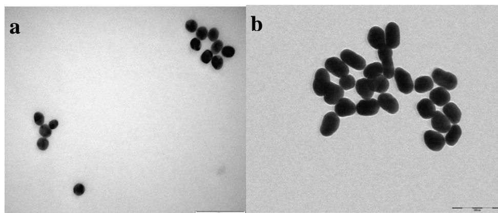
**Figure 2.1** TEM images of gold nanoparticles: **a** –AuNPs-T; **b** –AuNPs-F
