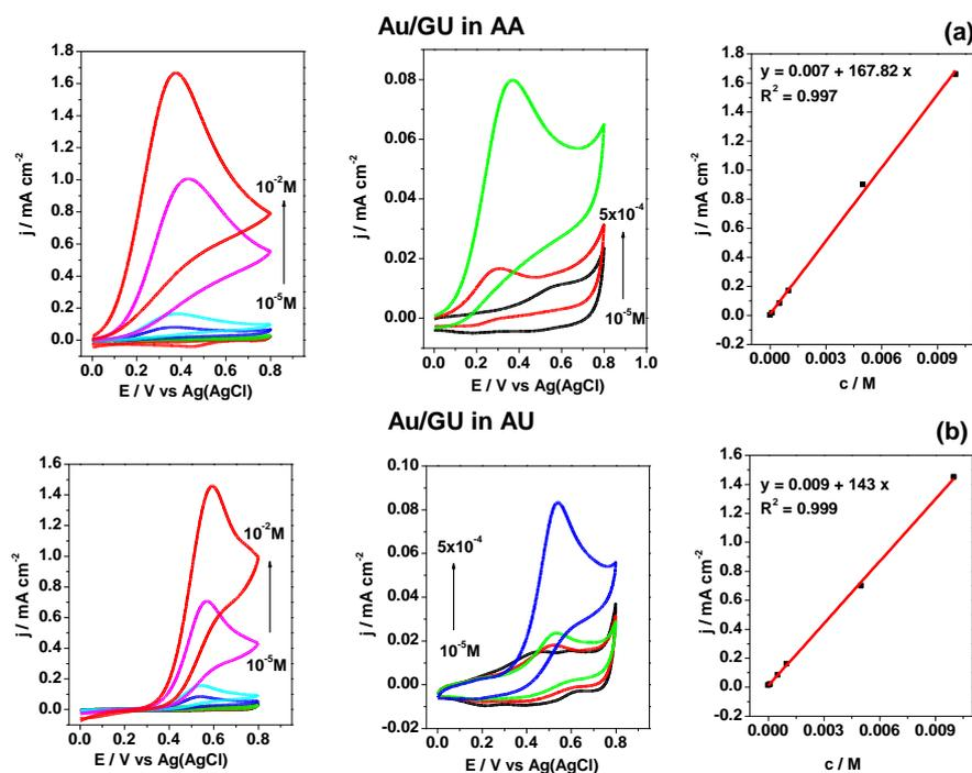
**Figure 3.6** Cyclic voltammograms recorded for **Au/GU** electrode in solutions containing ascorbic acid **(a)** or uric acid **(b)** and the corresponding calibration plots; scan rate 50 mV/s
