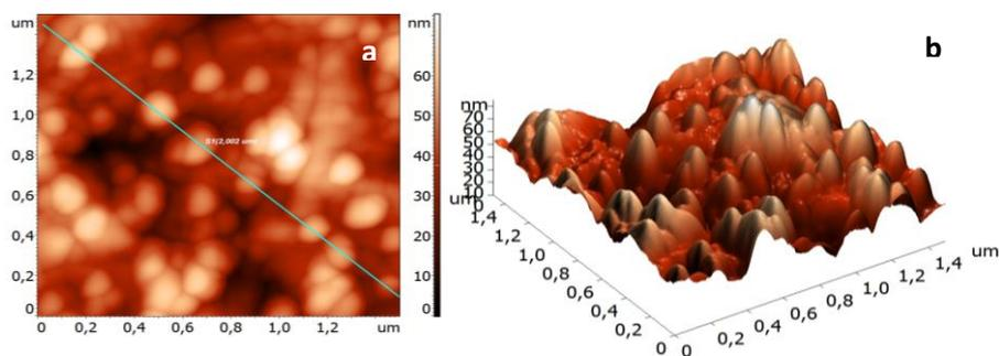
**Figure 2.17** AFM images of Au/TC/AuNPs-F electrode: **(a)** – 2D height image; **(b)** – 3D image
