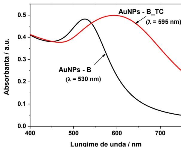
**Figure 2.6** UV-Vis spectra of AuNPs-B and AuNPs-B functionalized with thiocytosine (AuNPs-B\_T), 1:0.3 AuNPs-B:TC
