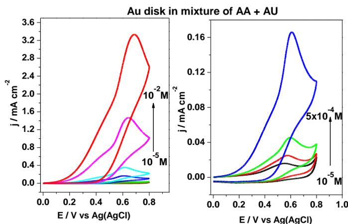
**Figure 3.11** Cyclic voltammograms recorded for **Au disk** electrodes in mixture of ascorbic and uric acid; scan rate 50 mV/s
