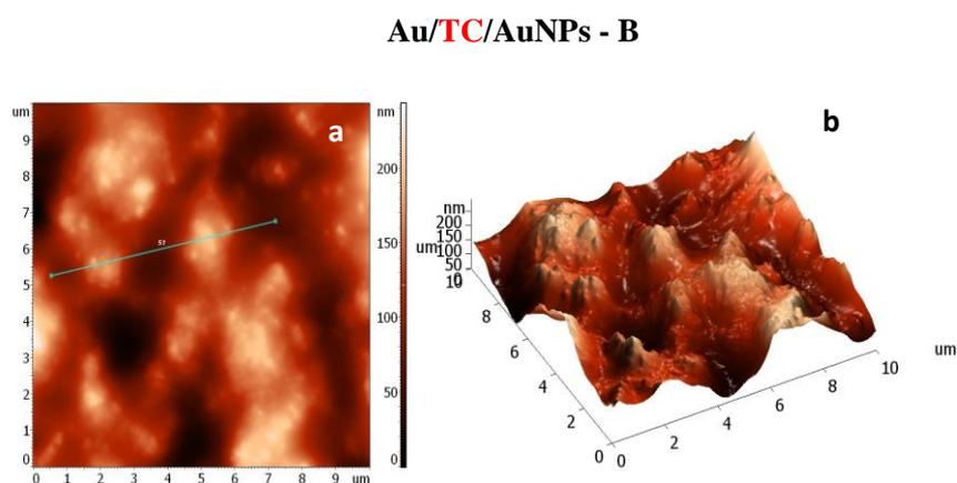
**Figure 2.19** AFM images for Au/TC/AuNPs-B electrode: **(a)** – 2D height image; **(b)** – 3D image
