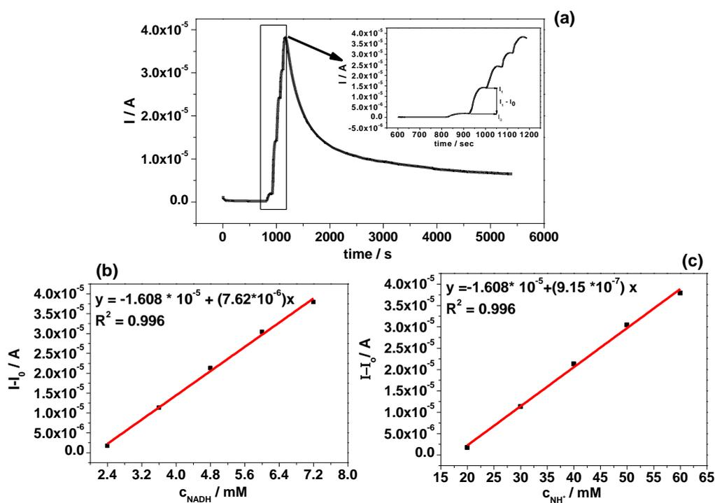
**Figure 4.8.** (a) Chronoamperogram obtained at Au/ TC/ AuNPs-F/ LeuDH modified electrode for successive addition of 1.2 mM NADH; (b) linear response in the 2.4 – 7.2 mM NADH concentration range; (c) indirect calibration plot of ammonium ion in the 20 – 60 mM concentration range;  $I_0$  – is background current
