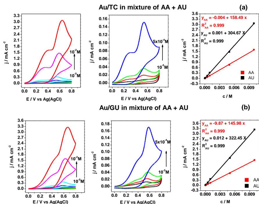
**Figure 3.12** Cyclic voltammograms recorded for Au/TC (a) and Au/GU (b) electrodes in solutions containing ascorbic and uric acid in mixture; the corresponding calibration plots; scan rate 50 mV/s
