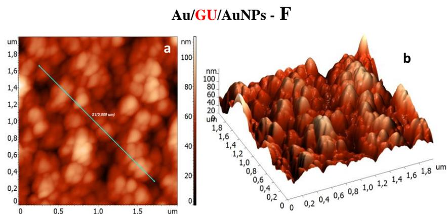
**Figure 2.18** AFM images of Au/GU/AuNPs-F electrode: **(a)** – 2D height image; **(b)** – 3D image
