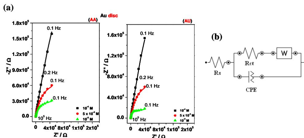
**Figure 3.13 (a)** Nyquist plots for Au disk electrode in PBS solution containing various ascorbic acid/ uric acid concentrations; the continuous lines represent the fit based on the equivalent circuit (b)
