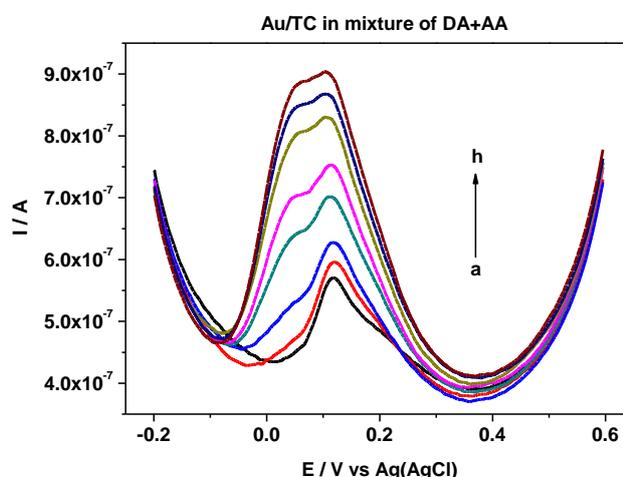
**Figure 3.16** DPVs recorded for Au/TC electrode in pH 7.2 PBS containing DA (5  $\mu\text{M}$ ) and AA – successive addition: a) 0, b) 5, c) 5, d-h) 10  $\mu\text{M}$
