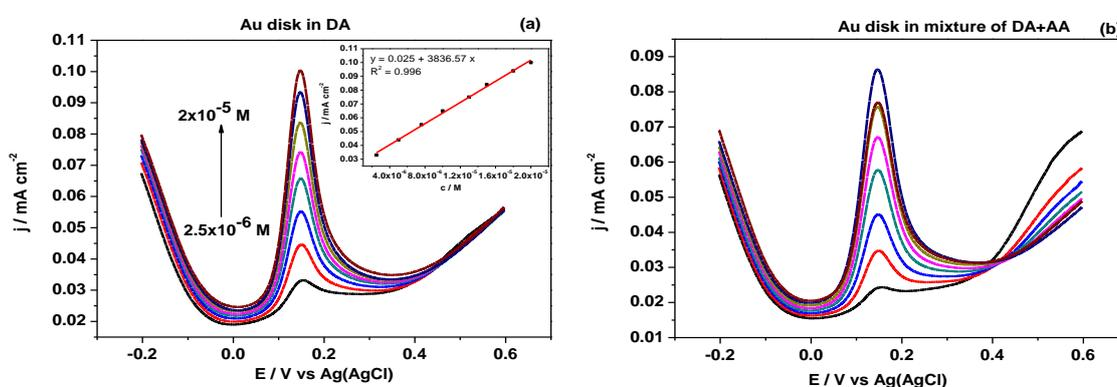
**Figure 3.15 (a)** DPVs recorded for Au disk electrode in pH 7.2 PBS containing DA:  $2.5 \times 10^{-6}$  M –  $2 \times 10^{-5}$  M, **inset:** linear response in concentration range  $2.5 \times 10^{-6}$  M –  $2 \times 10^{-5}$  M; **(b)** DPVs recorded for Au disk electrode recorded in solutions containing DA (successive addition of 2.5  $\mu\text{M}$ ) and AA (successive addition of 6.5  $\mu\text{M}$ )
