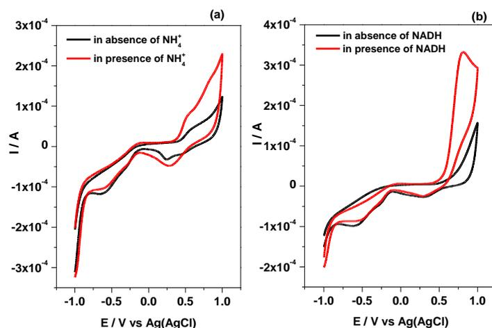
**Figure 4.7** Cyclic voltammograms of Au/TC/AuNPs/LeuDH modified electrode, in the absence and presence of 60mM  $\text{NH}_4^+$  ion (a) and in the absence and presence of 7.2 mM NADH (b) at pH 8; 50 mV/s scan rate
