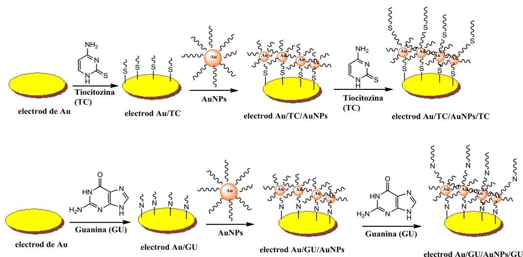
**Figure 3.1** Schematic illustration of modified electrodes preparation
