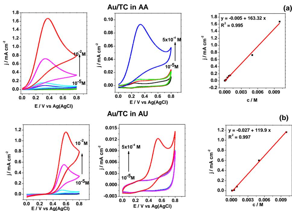
**Figure 3.5** Cyclic voltammograms recorded for **Au/TC** electrode in solutions containing ascorbic acid **(a)** or uric acid **(b)** and the corresponding calibration plots; scan rate 50 mV/s
