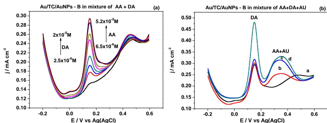
**Figure 3.19 (a)** DPVs recorded for Au/TC/AuNPs-B electrode in solutions containing DA (successive addition of 2.5  $\mu\text{M}$ ) and AA (successive addition of 6.5  $\mu\text{M}$ ); **(b)** DPVs recorded for Au/TC/AuNPs-B electrode in solutions containing DA: a-c) 20  $\mu\text{M}$ , d) 50  $\mu\text{M}$ ; AA: a-d) 52  $\mu\text{M}$  and AU: a) 0, b) 50, c-d) 100  $\mu\text{M}$
