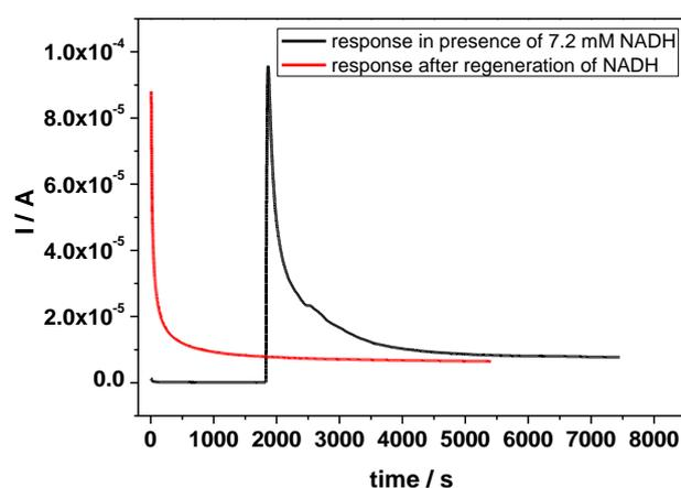
**Figure 4.12** Chronoamperograms obtained at Au/TC/AuNPs-F/LeuDH modified electrode in the presence of 7.2 mM NADH (black line) and after NADH regeneration (red line)
