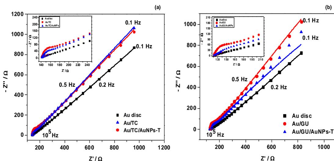
**Figure 2.15 (a, b).** Nyquist plots for: Au disk, Au/TC, Au/TC/AuNPs, Au/GU, Au/GU/AuNPs electrodes. The experiments were recorded in Zobel solution (0.003 M  $K_3Fe(CN)_6$  and 0.003 M  $K_4Fe(CN)_6$  in 0.1 M KCl), at an applied potential of +0.3 V vs Ag/AgCl; the continuous lines represent the fit based on the equivalent circuit
