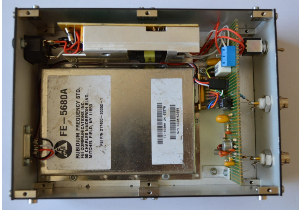
Figure 11: Rubidium Atomic Frequency Standard FE 5680A used in the experimental setup
