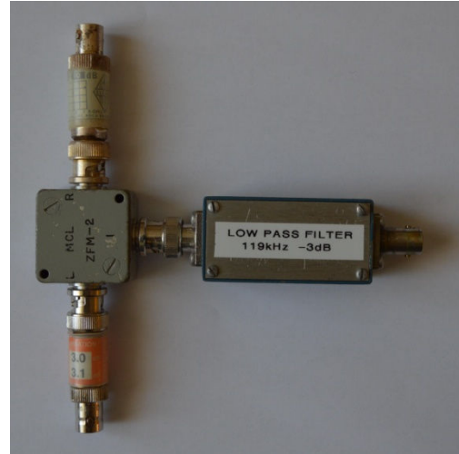
Figure 8: Low Pass Filter in its casing connected to the ZFM-2 passive mixer
