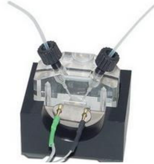
Figure 6: The used flow cell kit (model no. 011121)
