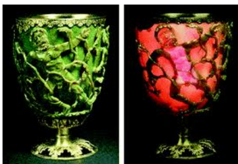
Figure 1-1 The Lycurgus roman cup which appears green in reflected light (left) and ruby-red in transmitted light (right) due to the presence of gold nanoparticles.
