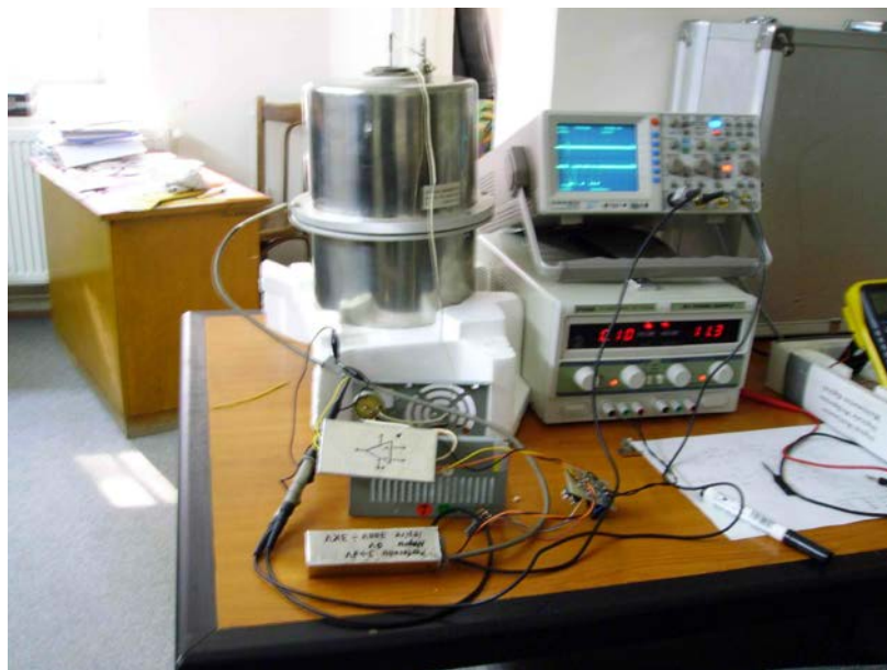
Fig. 2.18. Laboratory stand for tests by means of the ionisation chamber
