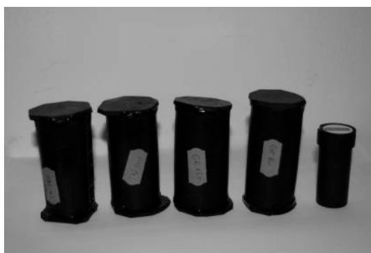
Fig. 3.32. CR 39 transducers placed in the basement (original)
