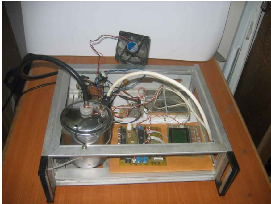
Fig. 2.19. Device with a ionisation chamber for measuring the radon concentration – inside view (original)
