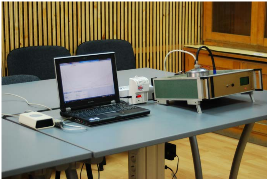
Fig. 2.20. Device with a ionisation chamber for measuring the radon concentration, during tests, alongside a Safety Siren 2 device and a Geiger Muller meter (original)
