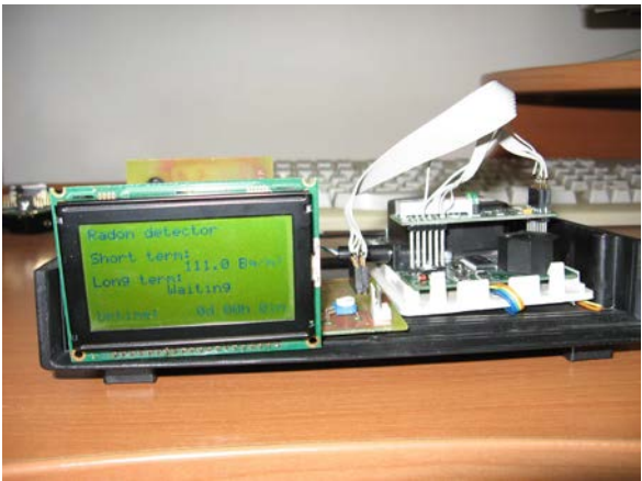
Fig. 2.16. Device with a detection chamber for measuring the radon content in the air (front view) (original)
