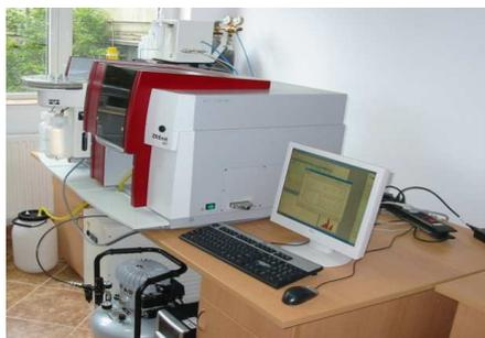
**Fig. 7.2. Zeenat 700 atomic absorption spectrometer**
