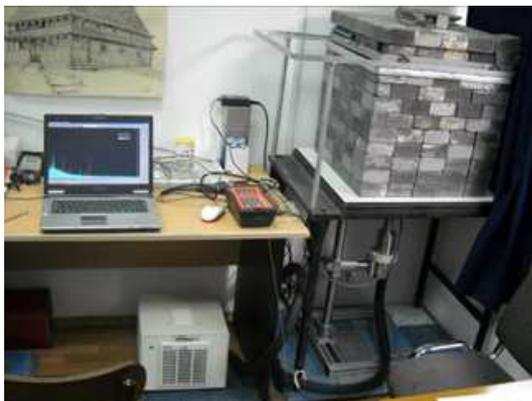
*Fig. 6.6. ORTEC GMX detector FWHM HpeGe 1.92KeV at 1.33MeV with Be window.*
