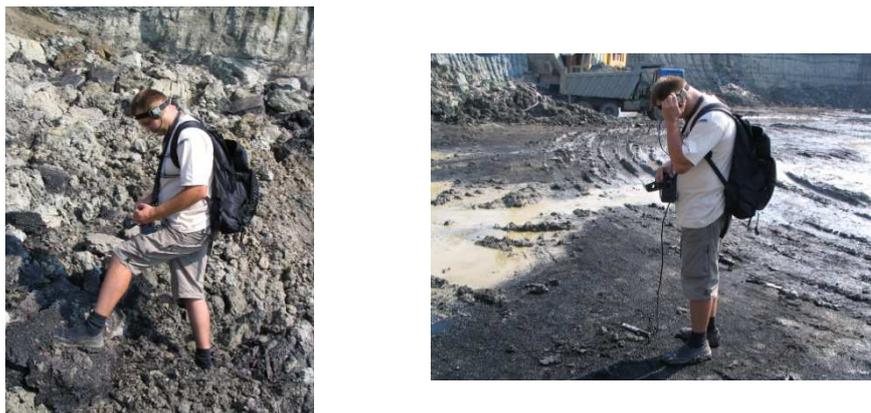
Fig. 6.1. Absorbed dose measurements made in Bobota II quarry/Sărmășag deposit
