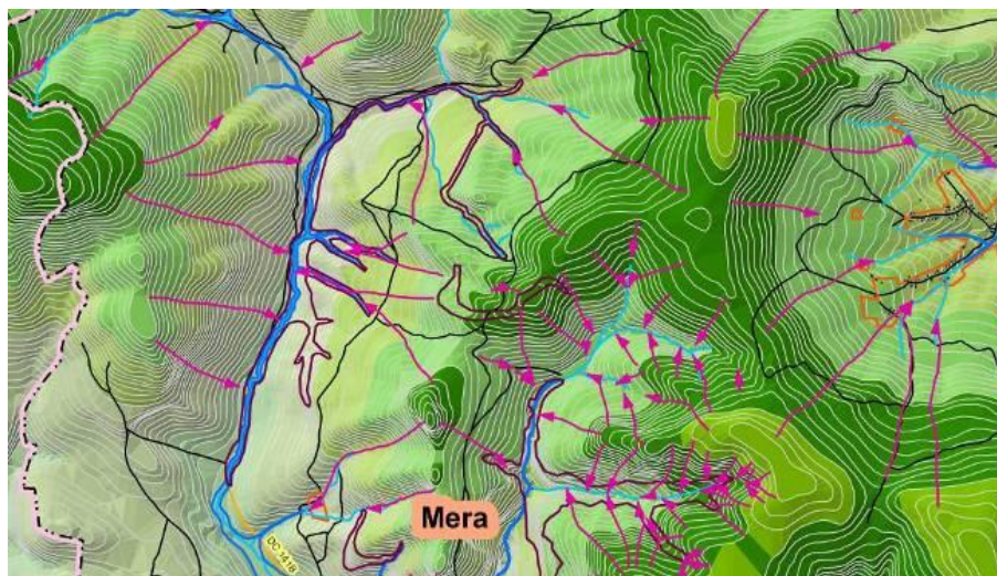
Figure 71. Leakage paths from hillsides identified for the Mera locality.
