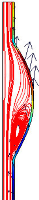
Figure 8.2 Artery with aneurysm. Stream lines and the displacement of the wall at a given time (non-Newtonian, viscoelastic model)
