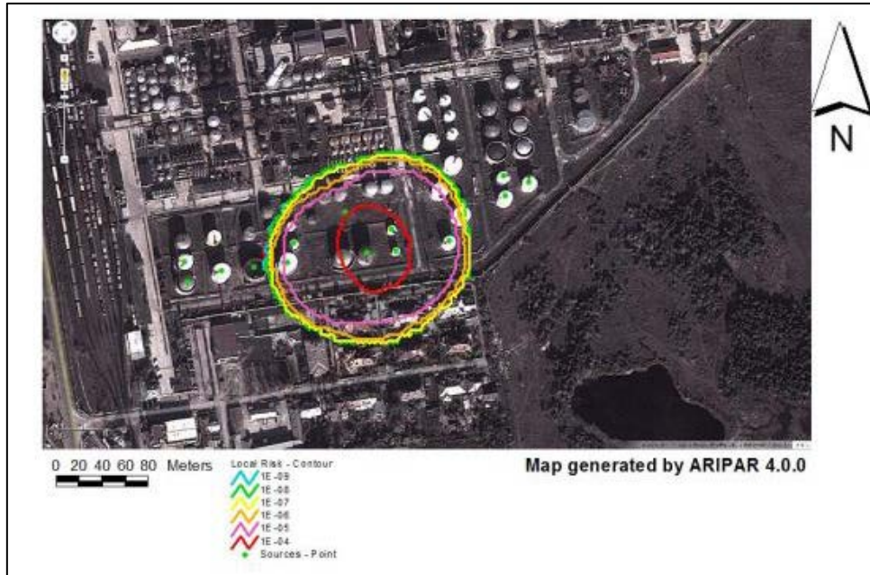
Figure 50a. Individual Risk map for tanks A7-A10 bund fire, intrinsic and seismic causes.
