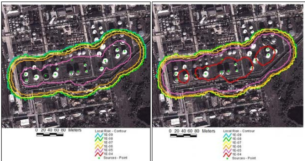
Figure 56. Side-by-side comparison of individual risk for fire in bund scenario for tanks A1-A15.
