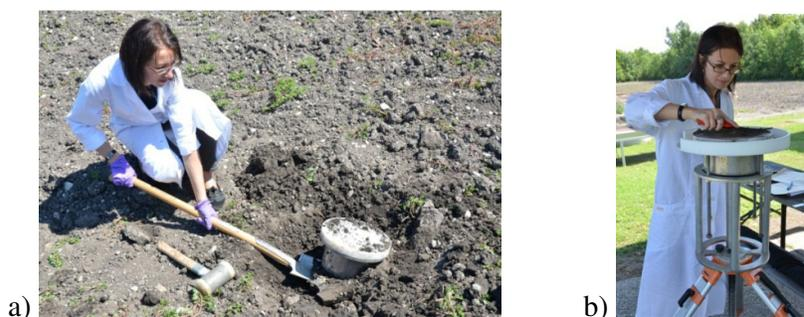
**Figure 7.** Soil core inside the stainless steel tube of the FSIC: (a) during sampling, and (b) during the incremental scraping
