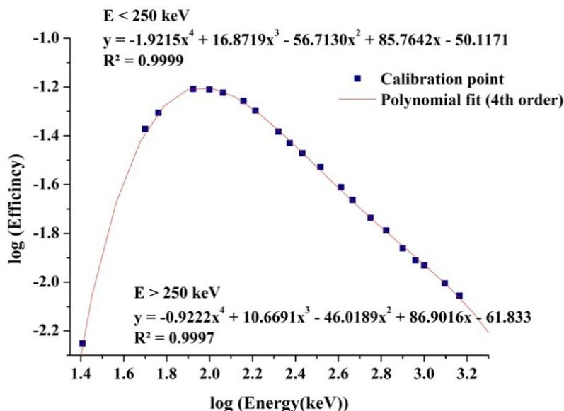
**Figure 14.** The efficiency curve of the Ortec GMX detector (25.5 – 1461 keV)
