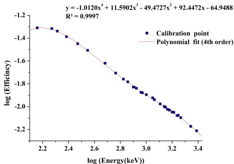
**Figure 13.** The efficiency curve of the Ortec GEM detector (144 – 2447 keV)
