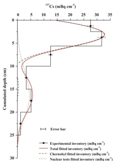
**Figure 3.** Experimental depth distribution of  $^{137}\text{Cs}$  in the reference site, Chernobyl and the nuclear tests fitting curves
