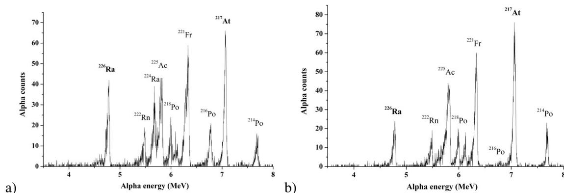
**Figure 9.** Alpha spectra of radium in a soil sample using  $^{225}\text{Ra}$  tracer and registered: (a) 3.7-8 days after the Ra/Th separation; (b) recounted about 17 days after separation
