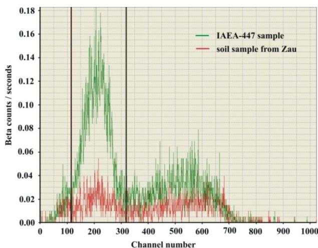
**Figure 10.** Beta spectrum of  $^{210}\text{Pb}$  with double window selection
