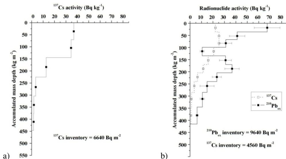
**Figure 1.** a)  $^{137}\text{Cs}$  depth distribution at the first reference site; b)  $^{137}\text{Cs}$  and  $^{210}\text{Pb}_{\text{ex}}$  depth distributions at the second reference site.
