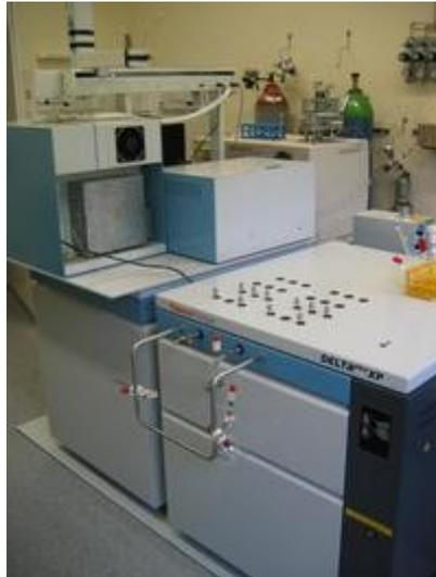
Figure 7.4 Thermo Finnigan Delta plus XP type stable isotope mass spectrometer
