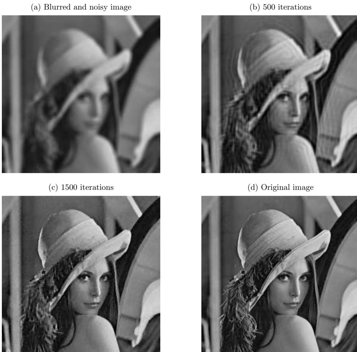
Figure 4.2: Figure (a) is the obtained image after multiplying with a blur operator and adding white Gaussian noise, (b) shows the averaged sequence generated by Algorithm 4.1.2 after 500 iterations. Figure (c) is the reconstructed image after 1500 iterations, (d) shows the clean  $256 \times 256$  Lena test image.
