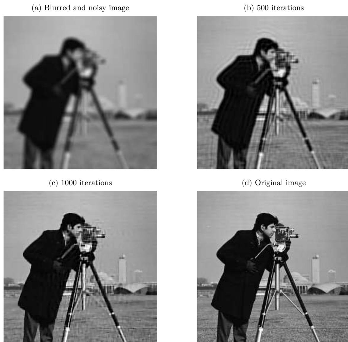
Figure 4.1: Figure (a) is the obtained image after multiplying with a blur operator and adding white Gaussian noise, (b) shows the averaged sequence generated by Algorithm 4.1.2 after 500 iterations. Figure (c) is the reconstructed image after 1000 iterations, (d) shows the clean  $256 \times 256$  Cameraman test image.
