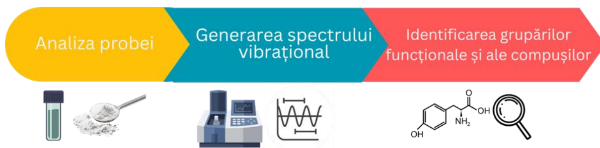
Figure 1.2. Workflow for IR spectral acquisition. Depending on the physical state of the sample, the analysis may be performed by direct placement on the ATR crystal, preparation of a KBr
