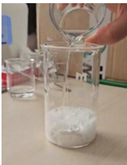
Figure 3.2.1. Rapid conversion reaction when phosphoric acid is dropped into biogenic carbonate with instant formation of brushite crystals (hydrated calcium phosphate mineral). Figure taken from: Bajama, I.; Maškarić, K.; Lazar, G.; Tamaş, T.; Costinaş, C.; Barbu-Tudoran, L.; Pinzaru, S.C. Aged Biogenic Carbonates from Crustacean Waste: Structural and Functional Evaluation of Calibrated Fine Powders and Their Conversion into Phosphate Minerals. Materials 2025, 18, 5119. https://doi.org/10.3390/ma18225119
