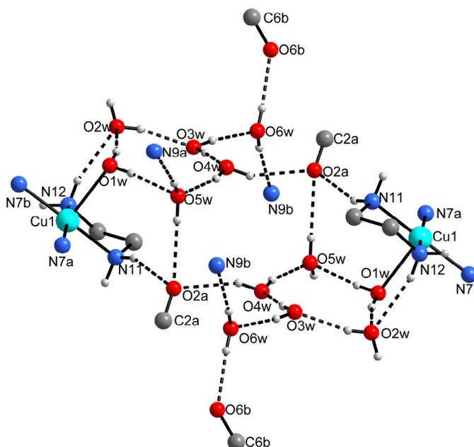
**Figure 12.** Extended hydrogen bonding interactions between two  $\text{Cu}(\text{dphen})$  units in **18**, realized through  $\{\text{H}_2\text{O}\}_5$  rings and oxygen atoms of  $\text{C}2\text{a}(\text{O}2\text{a})$  carbonyl groups
