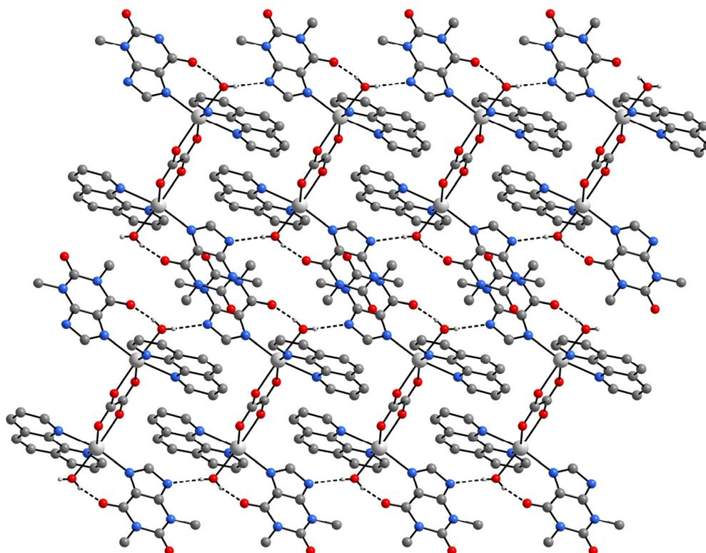
**Figure 17.** Twodimensional hydrogen bond network packing of **24**, viewed along  $b$  axis
